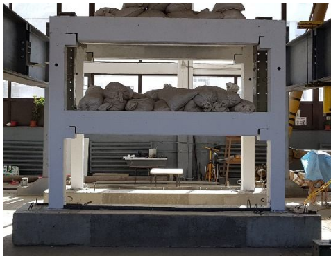
Fig. 2 – First test on Experimental Frame: Non stiffened 2014.
