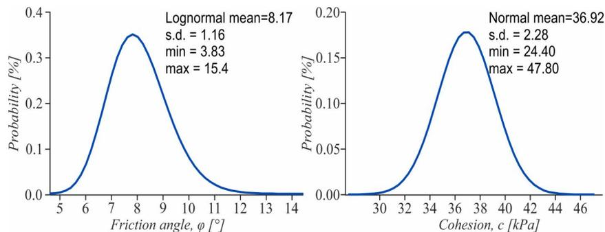
Fig. 3 – Probability density functions for friction angle and cohesion.
