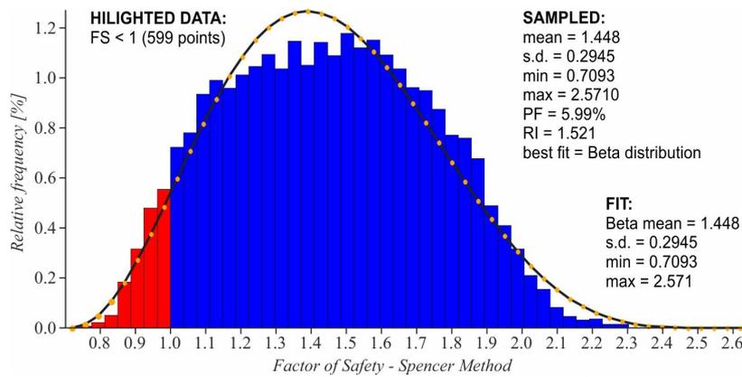
Fig. 9 – Results of slope stability analyses using Eurocode 8 (seismic conditions).
