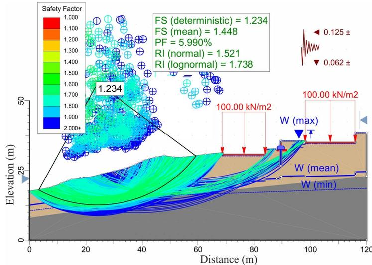
Fig. 8 – Results of probabilistic slope stability analyses.
