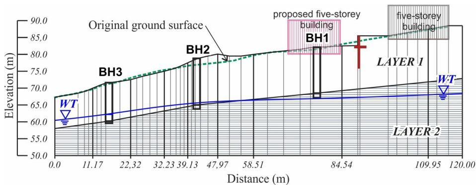
Fig. 2 – Slope profile at Section A-A.
