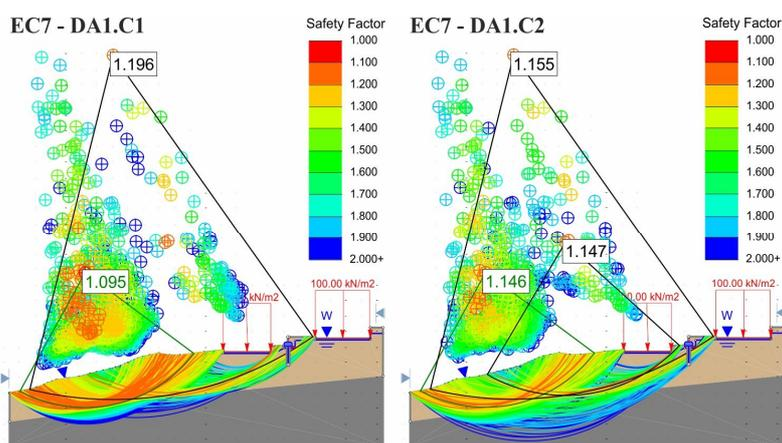
Fig. 6 – Results of semi-probabilistic slope stability analyses under static conditions with water table located on slope surface.
