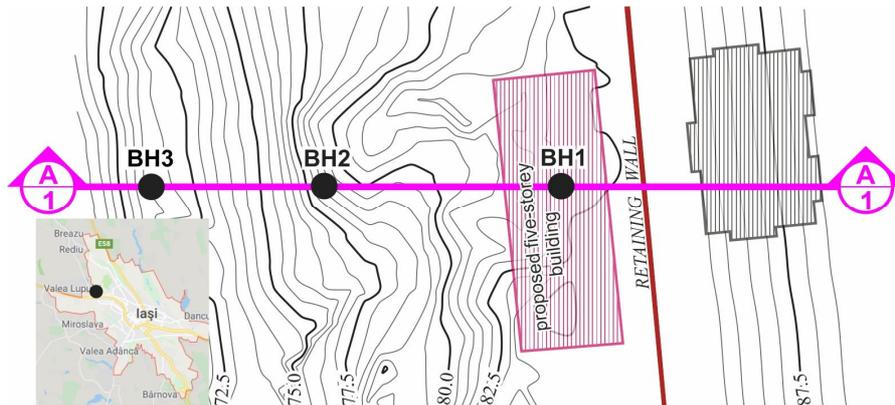
Fig. 1 – Plan view of the slope with boreholes' locations.
