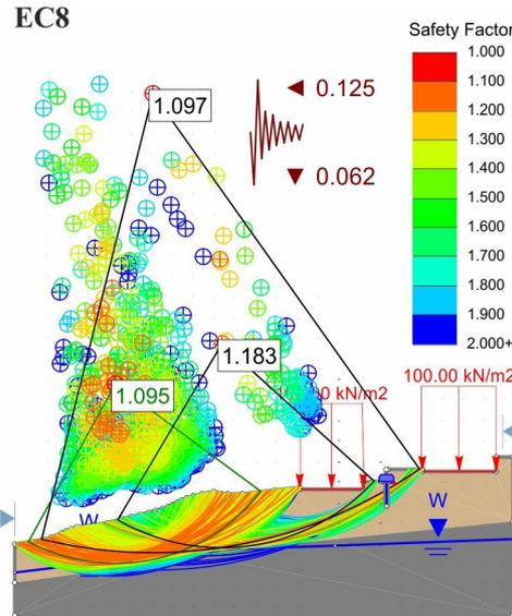
Fig. 7 – Results of semi-probabilistic slope stability analyses under seismic conditions.
