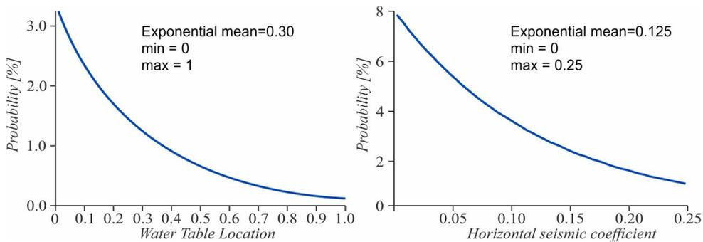
Fig. 4 – Probability density functions for water table location and horizontal seismic coefficient.
