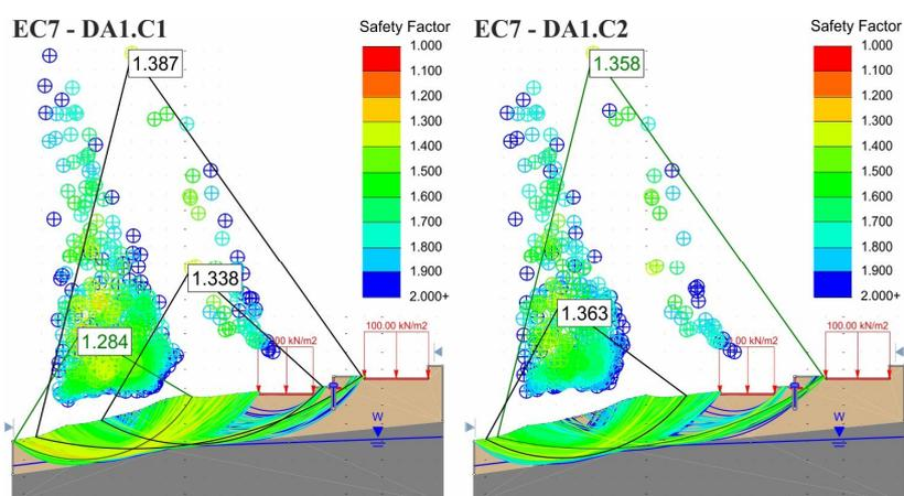
Fig. 5 – Results of semi-probabilistic slope stability analyses under static conditions with current water table.
