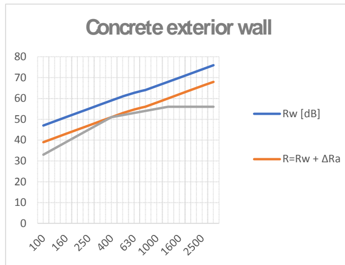
Fig. 2 – Sound reduction index curve R_i(f) – reinforced concrete wall.
