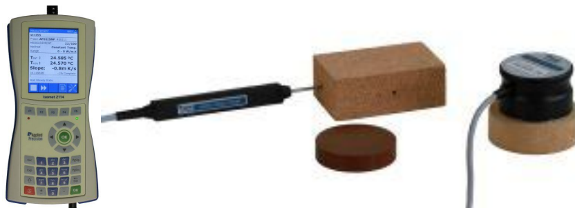
Fig. 2 – Measuring device ISOMET 2114.
