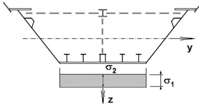
Fig. 10 – Shear lag effect in tension flange.
