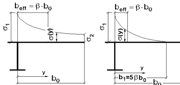
Fig. 4 – Distribution of stresses due to shear lag (SR EN 1993-1-5: 2006).
