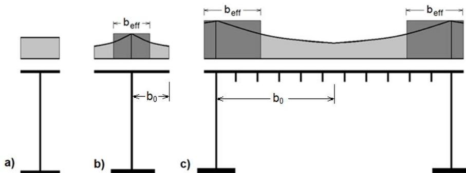
Fig. 1 – Effective width due to shear lag: a) thin wide flange; b) wide flange; very wide flange.
