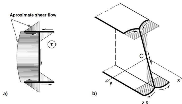
Fig. 2 – a) Shear flow due to a vertical shear  $V_z$ ; b) Warping displacement due to shear. (Trahair *et al.*, 2008).
