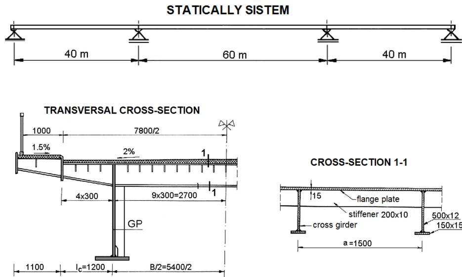
Fig. 5 – Steel bridge analyzed.
