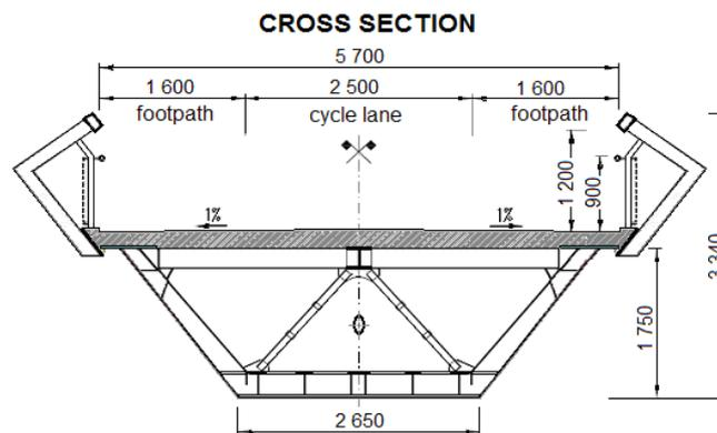
Fig. 8 – Pedestrian bridge cross-section.
