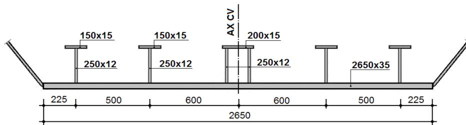
Fig. 9 – Bottom flange for the central segment.
