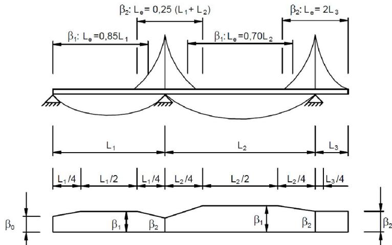
Fig. 3 – Definition of the effective length  $L_e$  (SR EN 1993-1-5: 2006).
