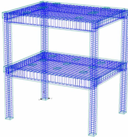
Fig. 3 – Representation of the reinforcement mode of the analytical representative RC moment-resisting frame model (ATENA software).
