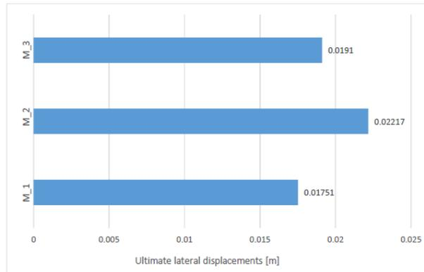
Fig. 5 – Influence of concrete strength class on the ultimate lateral displacement for M\_1, M\_2 and M\_3 models.
