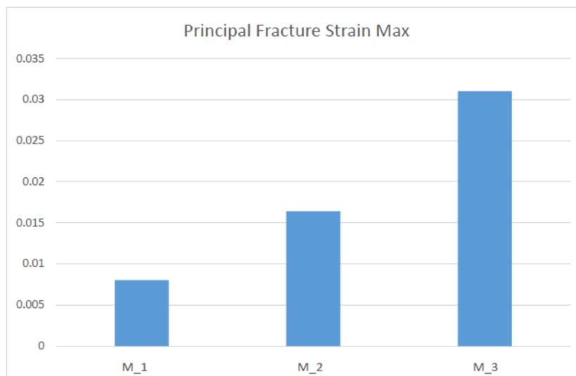
Fig. 9 – Influence of concrete strength class on the principal fracture strains for the M\_1, M\_2 and M\_3 models.
