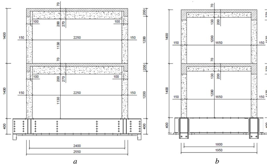
Fig. 2 – Geometry of the RC moment-resisting frame models: (a) global longitudinal section; (b) global transverse section – dimensions in mm.
