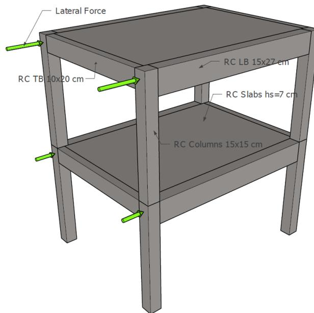
Fig. 4 – Direction of lateral forces application of the analytical representative RC moment-resisting frame model.
