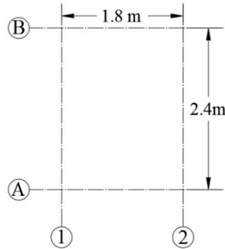
Fig. 1 – The inter-axis distance for RC moment-resisting frame models.
