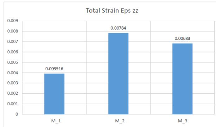
Fig. 7 – Influence of concrete strength class on the axial strain in columns for the M\_1, M\_2 and M\_3 models.
