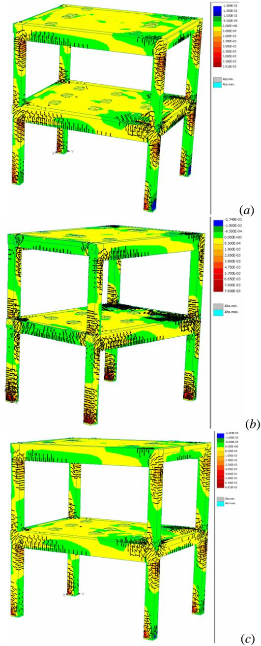
Fig. 8 – Eps<sub>zz</sub> strain for: (a) M\_1; (b) M\_2; (c) M\_3 RC moment-resisting frame models, ultimate step of lateral loading.
