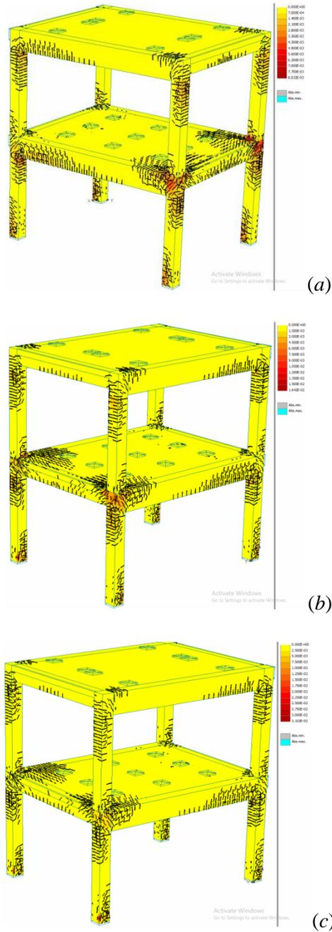
Fig. 10 – Principal fracture strain max for: (a) M\_1; (b) M\_2; (c) M\_3 models, ultimate step of lateral loading.
