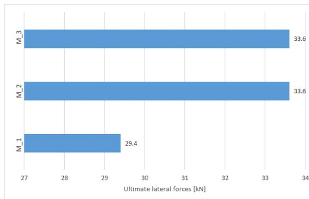
Fig. 6 – Influence of concrete strength class on the ultimate lateral loads for the M\_1, M\_2 and M\_3 models.
