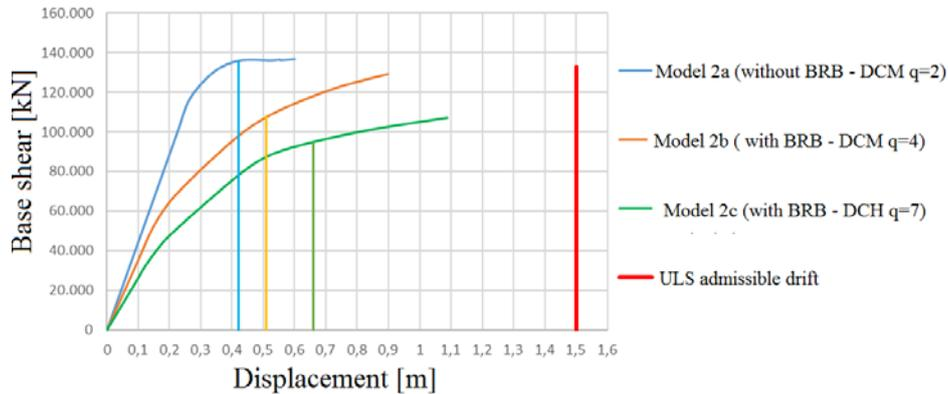
Fig. 6 – Push-over curves for 2a,2b and 2c models on X direction.
