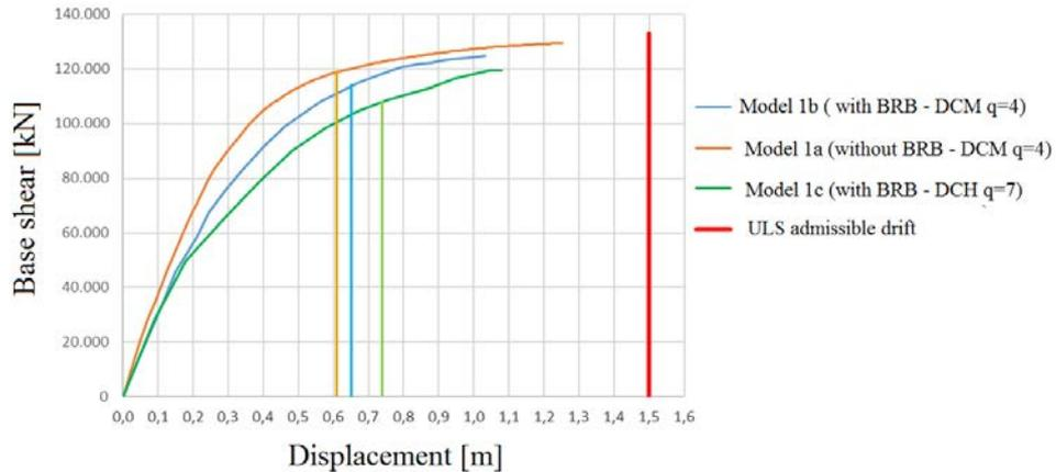
Fig. 5 – Push-over curves for 1a,1b and 1c models on X direction.
