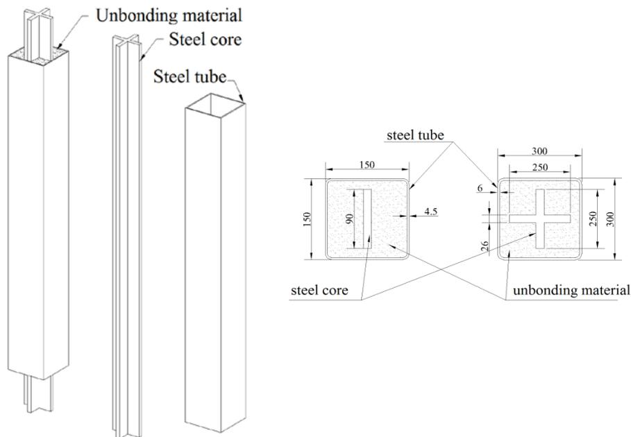
Fig. 1 – BRB types used in structural analysis (Black *et al.*, 2002).
