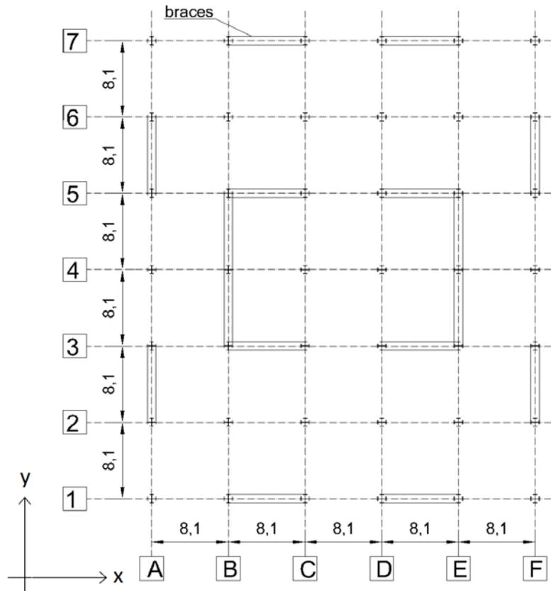
Fig. 3 – Structure layout (Ionescu-Lupeanu and Dima, 2017).
