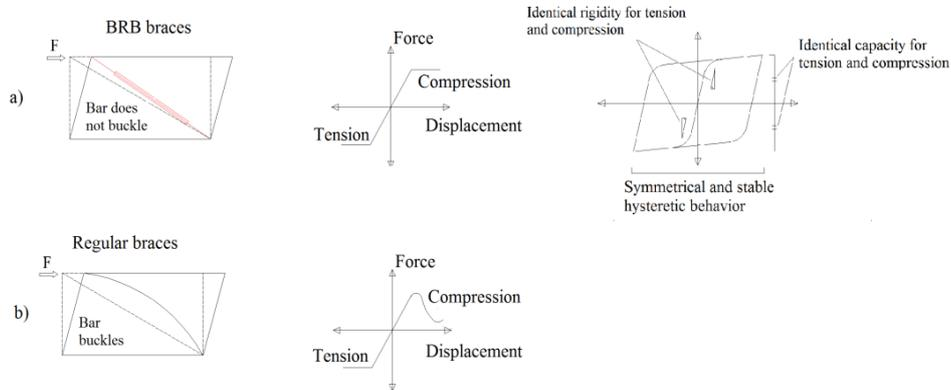
Fig. 2 – a) behaviour of BRB; b) behaviour of regular braces.
