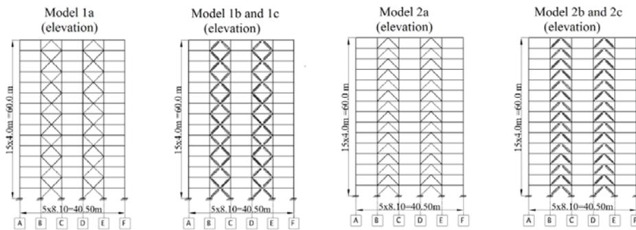
Fig. 4 – Models elevations (Ionescu-Lupeanu and Dima, 2017).
