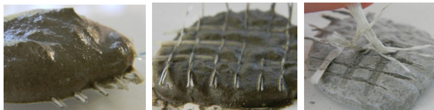
Fig. 7 – Mineral matrix with unidirectional mesh.
