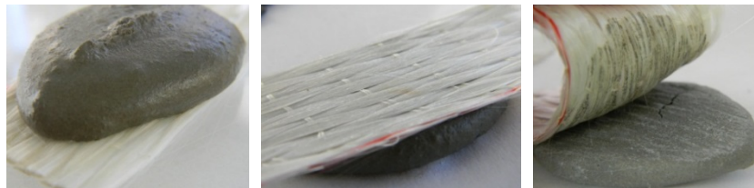
Fig. 4 – Mineral matrix with unidirectional reinforcement.
