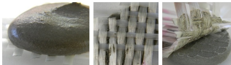
Fig. 5 – Mineral matrix with bidirectional reinforcement with no mails.
