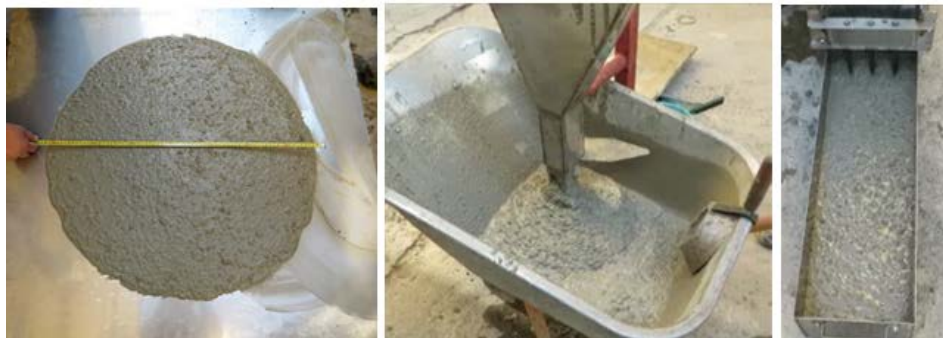
Fig. 1 – Testing SCC workability.
