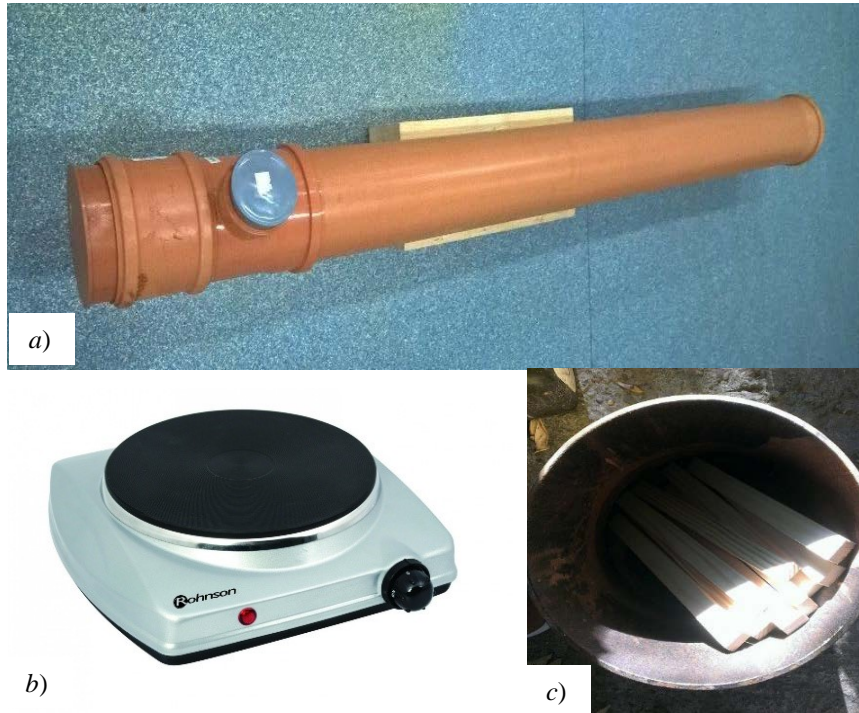
Fig. 5 – a) PVC container provided with a filling hole and an overflow hole; b) 220 V electric hob; c) specimens left to cure in a metal vessel.
