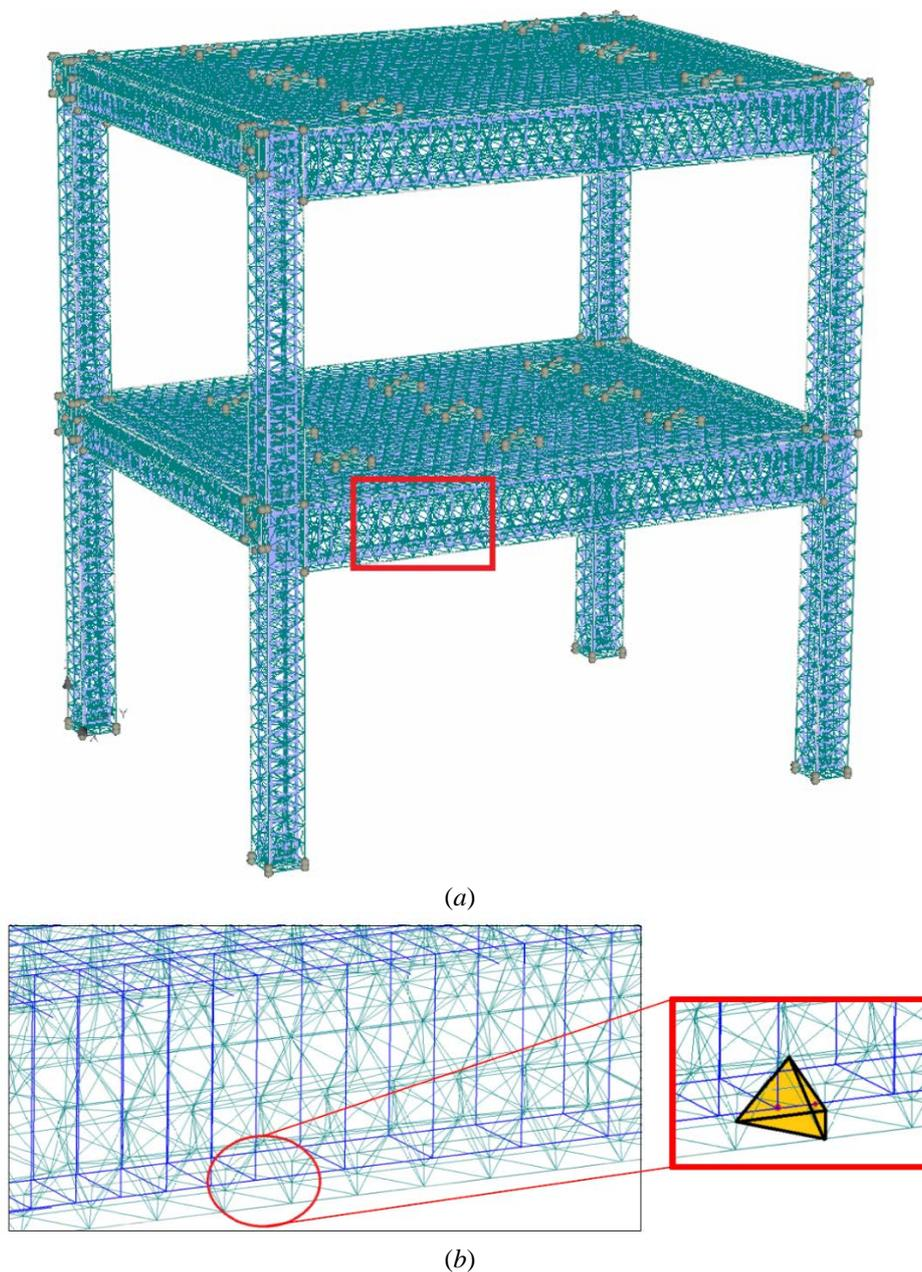
Fig. 2 – Graphic representation of coupling finite elements with demonstration of interaction between steel reinforcements and concrete for M<sub>5</sub> RC frame model: (a) 3D total mesh discretization; (b) Local representation of rebars – concrete interaction (ATENA software, 2015; Mihai *et al.*, 2007; Bitencourt Jr. *et al.*, 2018).
