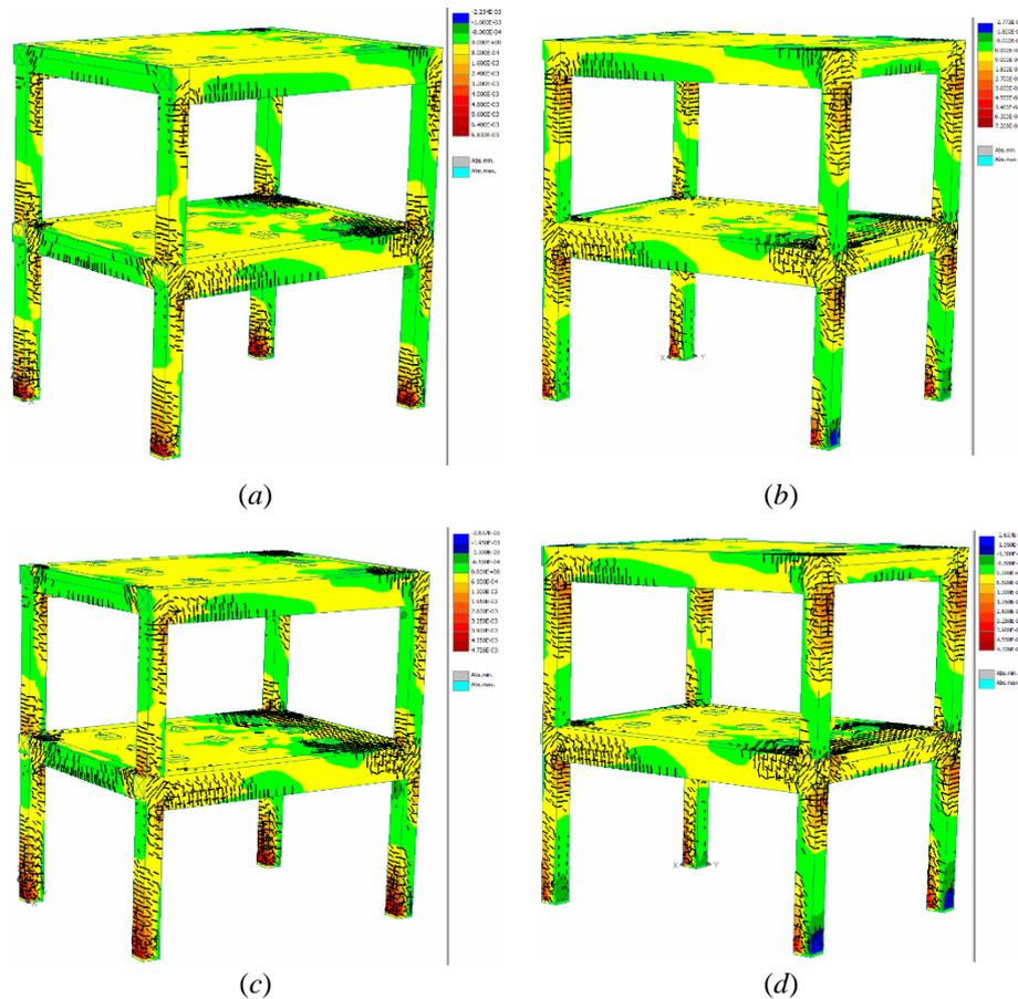
Fig. 6 – Total Strains  $\epsilon_{zz}$  (TSE) for: (a) M\_3; (b) M\_4; (c), (d) M\_5 moment resisting RC frame systems (models) in the case of the ultimate lateral loading step (see Table 1, Table 2 and Fig. 5).
