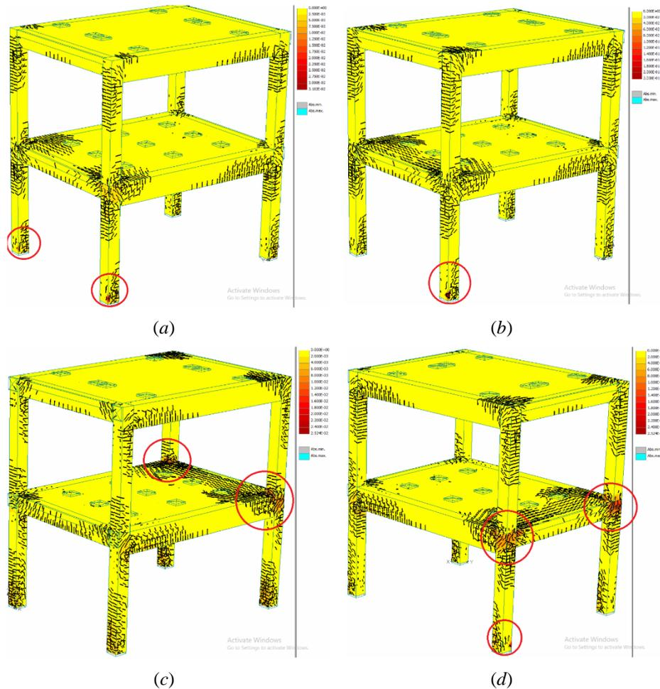
Fig. 8 – Principal Fracture Strains Max (PFSM) for: (a) M\_3; (b) M\_4; (c), (d) M\_5 moment resisting RC frame systems (models) in the case of the ultimate lateral loading step (see Table 1, Table 2 and Fig. 7) (Note: in the red circles are registered the maximum values of the PFSM).
