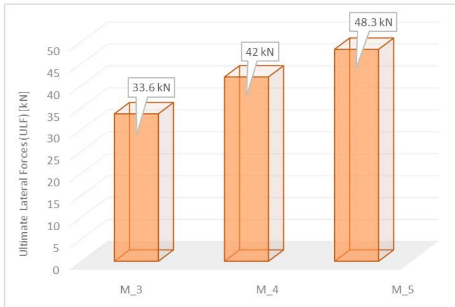
Fig. 4 – Influence of longitudinal steel reinforcement ratio in the RC columns on the Ultimate Lateral Forces (ULF) response of the M\_3, M\_4 and M\_5 RC moment resisting frame systems (see Table 1 and Table 2).
