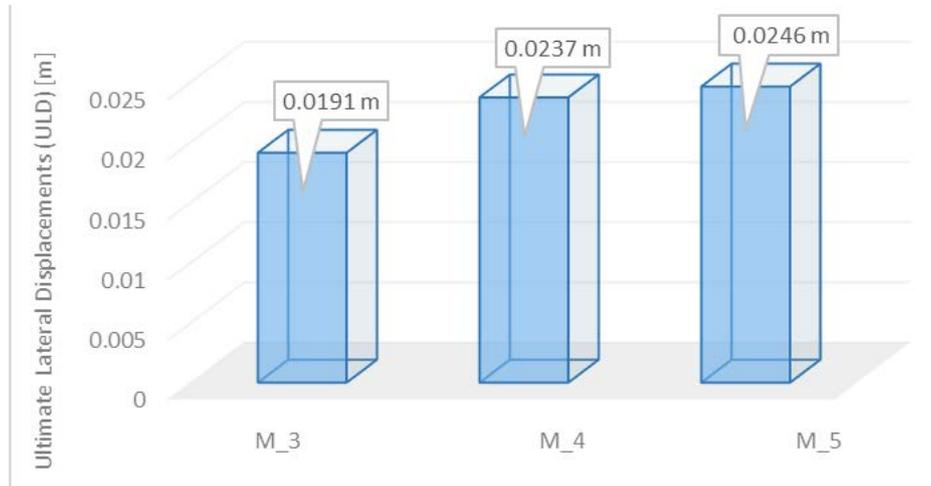
Fig. 3 – Influence of longitudinal steel reinforcement ratio in the RC columns on the Ultimate Lateral Displacements (ULD) response of the M\_3, M\_4 and M\_5 moment resisting RC frame models (see Table 1, Table 2).
