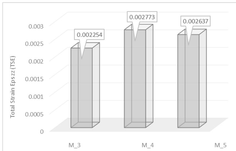
Fig. 5 – Influence of longitudinal steel reinforcement ratio in the RC columns on the lateral (seismic) response in **T**otal **S**trains **E**ps zz (TSE) of the M\_3, M\_4 and M\_5 moment resisting RC frame systems (general informations: Table 1 and Table 2).
