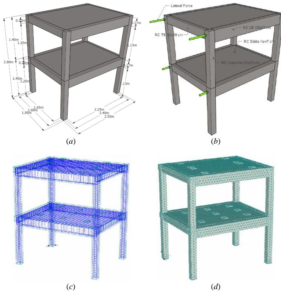
Fig. 1 – (a) General dimensions of the RC moment resisting frame models with longitudinal rigid beams; (b) Lateral static loading consideration mode for pushover performing of the RC frame models (Sococol *et al.*, 2020); (c) Steel reinforcement positioning in RC frame models (or representative RC frame model) (Sococol *et al.*, 2020); (d) Total mesh discretization of structural elements (ATENA software, 2015; Mihai *et al.*, 2007).
