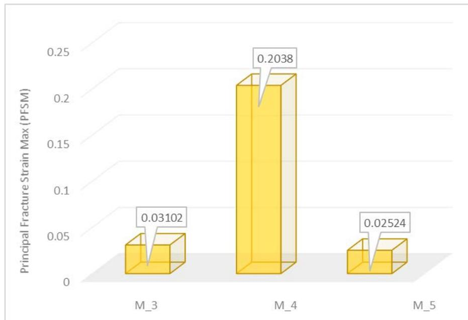
Fig. 7 – Influence of longitudinal steel reinforcement ratio in the RC columns on the lateral (seismic) response in Principal Fracture Strains Max (PFSM) of the M\_3, M\_4 and M\_5 moment resisting RC frame systems (models) (see Table 1 and Table 2).
