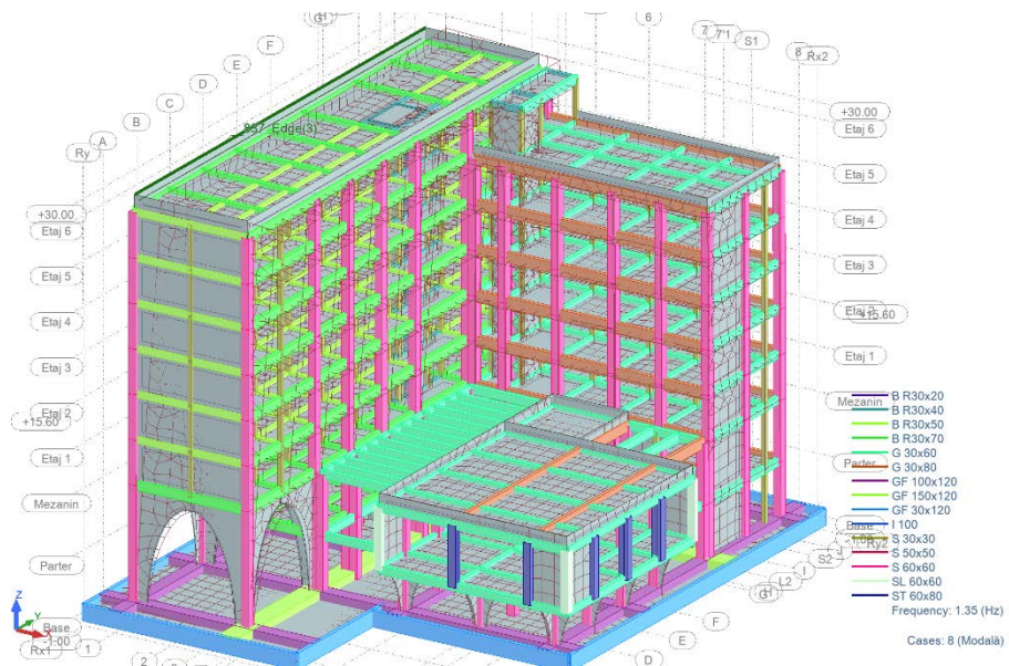
Fig. 13 – Vibration mode 4, F=1.35 Hz (mass participation 35.93% X; 3.02% Y).
