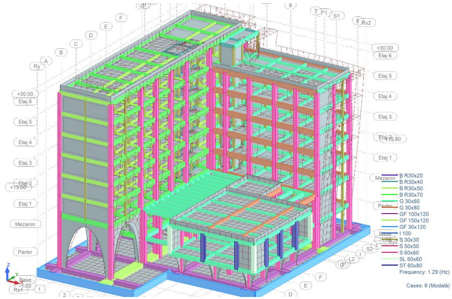
Fig. 12 – Vibration mode 3, F=1.29 Hz (mass participation 3.30% X; 44.63% Y).
