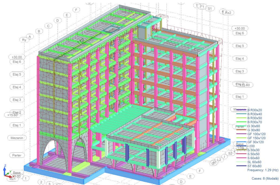
Fig. 11 – Vibration mode 2, F=1.29 Hz (mass participation 5.02% X; 0.24% Y).
