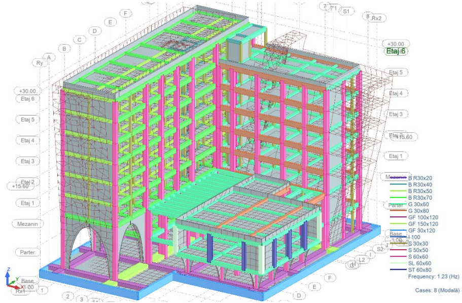
Fig. 10 – Vibration mode 1, F=1.23 Hz (mass participation 5.74% X; 1.79% Y).
