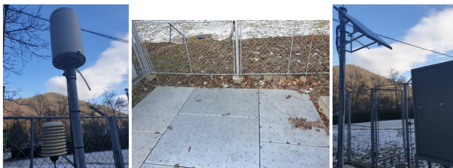
Fig. 9 – Automatic weather station (Cireșoaia) for measuring rainfall, temperature and snow layer mounted by WATMAN project.
