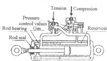
Fig. 1.– Semi-active fluid damper described by Karnopp.
