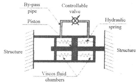
Fig. 2.– Scheme of variable orifice fluid damper.
