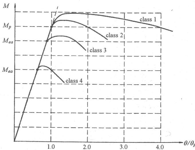
Fig. 1.- Moment *vs.* rotation dependence according to the cross section class.
