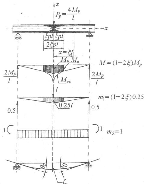
Fig. 5.– Elastic – plastic displacement for a simple supported beam.
