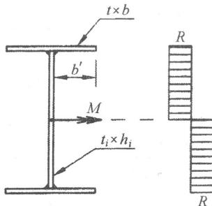
Fig. 2.– Bent element – distribution of stresses.
