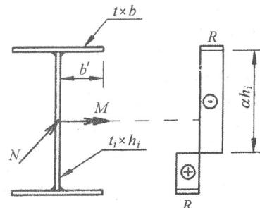
Fig. 3.– Compressed and bent element – distribution of stresses.
