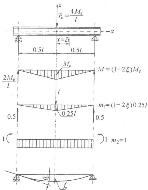
Fig. 4.– Elastic displacements for a simply supported member.
