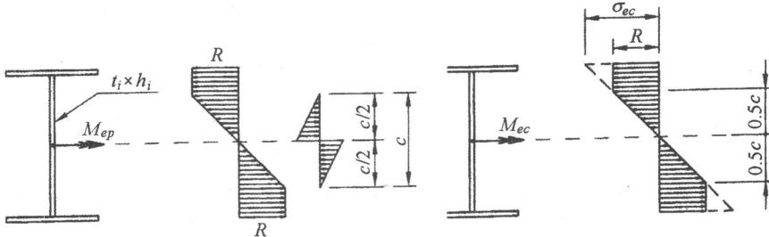
Fig. 6.- Distribution of stresses from the elastic-plastic bending moment.
